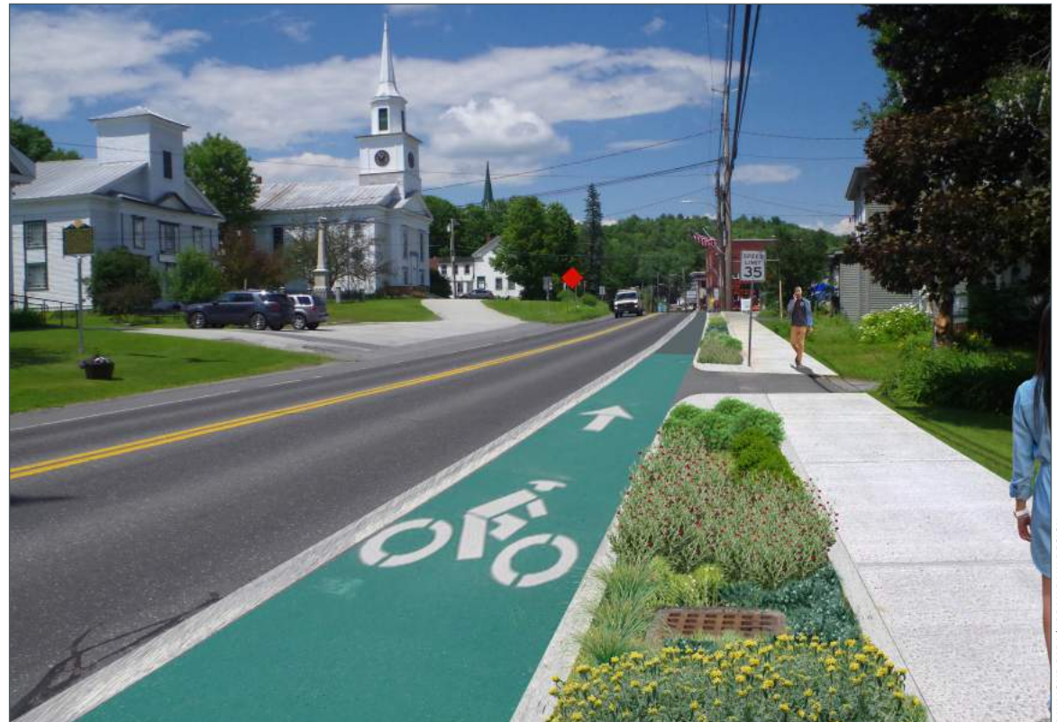
▲ RETROFIT OPPORTUNITY: The same arterial street retrofitted with a green gutter system, as well as additional street trees.
