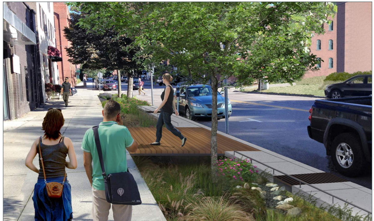
▲ RETROFIT OPPORTUNITY: The same downtown main street retrofitted with a series of stormwater planters.
