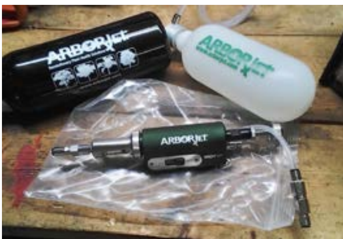
Ash injection system for EAB treatment.
